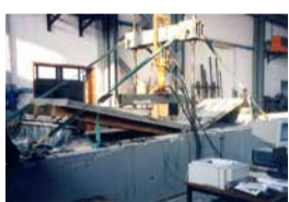
Test to break up the slab wood-concrete LPR connectors. A relevant fact that proves that the wealth of the Peter Cox technology is in the infinitely rigid behavior of the mixed section for macro deformations.
