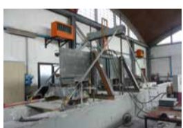
Test of mixed wood-concrete slab-laid concrete cutting to check the stiffness in the plane, which is essential to transmit the seismic force to the walls.
